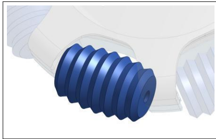
Fig. 2.4: Subwheel design with a tread pattern for better traction.
