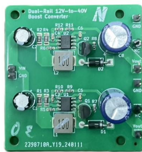
Fig. 9: First Prototype of Kicker Circuit
