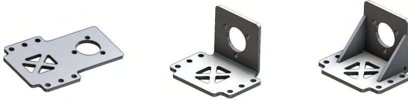
Fig. 6. Motor mount manufacturing process: from sheet metal to welding
