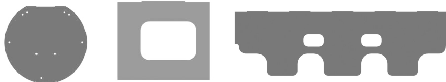
Fig. 2: The top, front and side part of our cover in order from left to right as they are cut out by the laser
