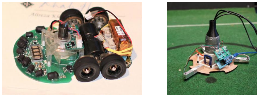
(a) MicroMouse with suction fan [4].
