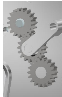
Fig. 6. Triple gear system for the dribbler.
