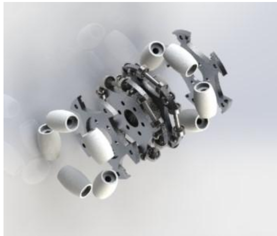
Fig. 4. Exploded view of designed omni-wheel
