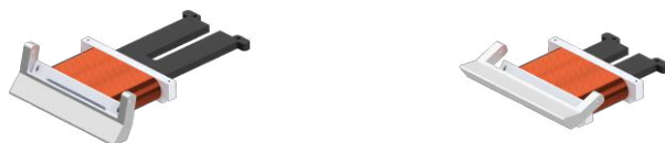
Fig. 2: Principle of Operation. The left picture shows the rest position of the plunger. In the right image, the plunger in its extended state is depicted.
