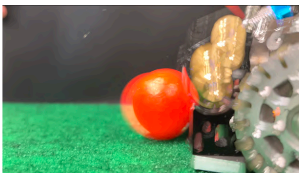
Figure3.7: Ver4.0 Dribbler hold accuracy
