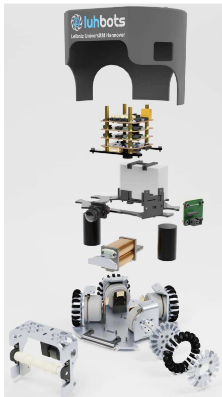
Fig. 2: Assembly of the first robot generation
