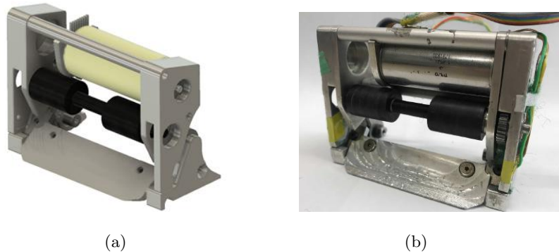
Fig. 3. Proposed dribbler (a)3D CAD image and (b)photo
