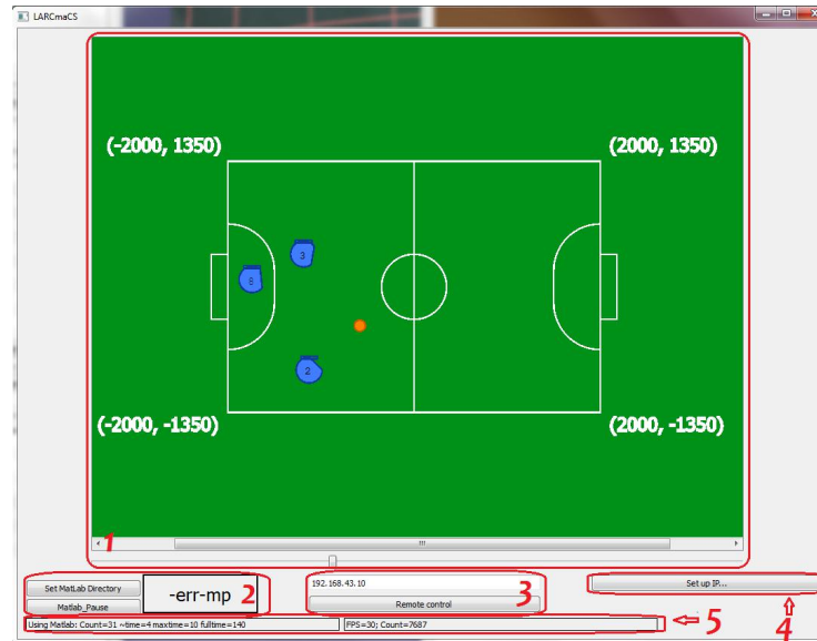
Fig. 2: Main window of our application. 1. Game Field 2. Matlab block 3. Remote control block 4. IP Settings 5. Information bars
