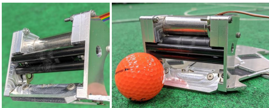
Fig. 3. Prototype dribbler used for the test.
