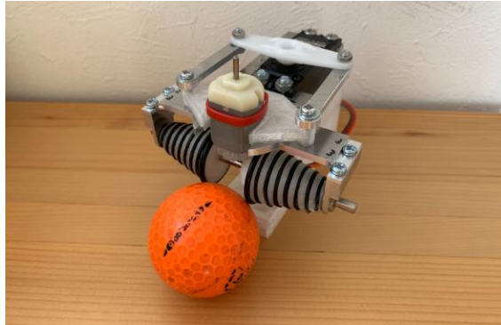
Fig. 6. Experimental prototype dribbler for the test.
