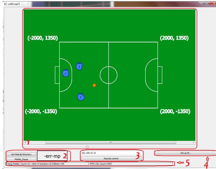
Fig. 6: Main window of our application. 1. Game Field 2. Matlab block 3. Remote control block 4. IP Settings 5. Information bars
