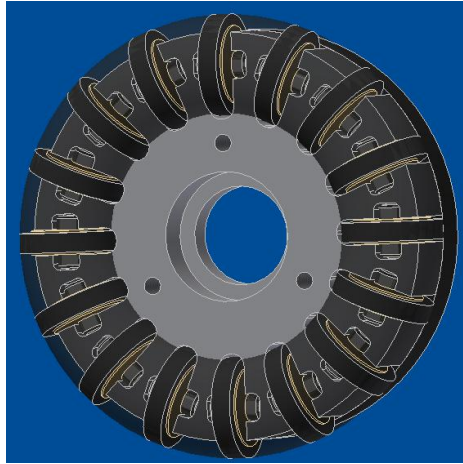
Fig. 1: Bearing pocket in the back-plate of the wheel
