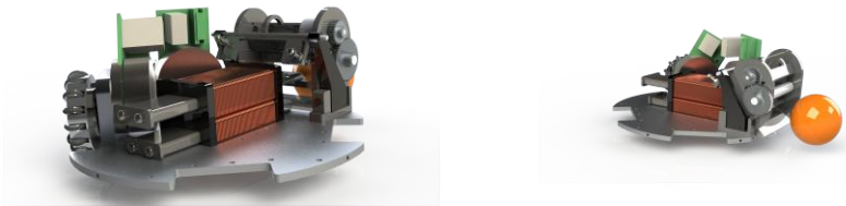
Fig. 2: Integrated views of straight kicker, chip kicker and dribbler
