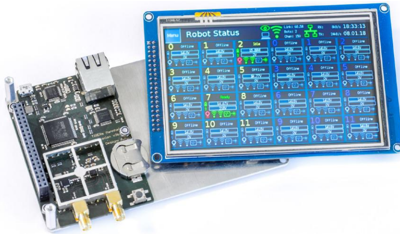
Fig. 2: Base Station v2018 with exemplary display content showing all robots and an info bar on top.
