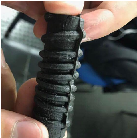
Fig. 8: Roller made with silicon rubber
