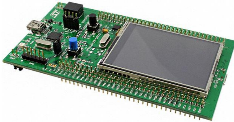
Fig. 2. STM32F429ZI Discovery Board.
