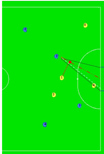
Fig. 11. This figure shows how one of the functions operates. At first, game plan notes that the opponent's robot wants to shoot the ball toward our goal, and then the game plan specifies that the nearest teammate robot to the opponent kicker is robot number 1. Therefore, this robot is responsible for blocking the kicker. When the game plan calls the function for robot number 1, the function finds the best position for the robot (according to the position of the opponent's robot and the ball) to prevent goal.
