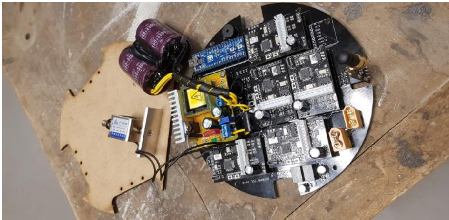
Fig. 4. The kicker circuit, the solenoid and the two capacitors
