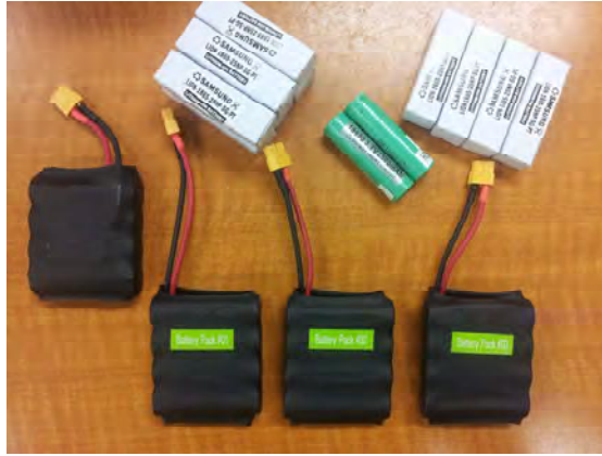
Fig. 9. Battery pack assembly beside individual cells
