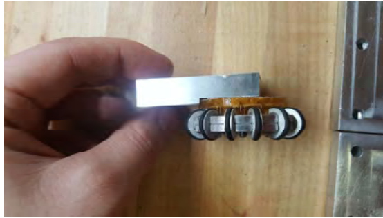
Fig. 5. View of the omni wheel-gear assembly.
