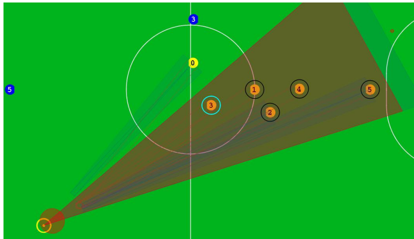
Fig. 7: Choosing the best robot to catch a rolling ball. The red triangle visualizes the direction of the pass. All robots with a black circle are potential receivers. The best robot is marked with a cyan circle.
