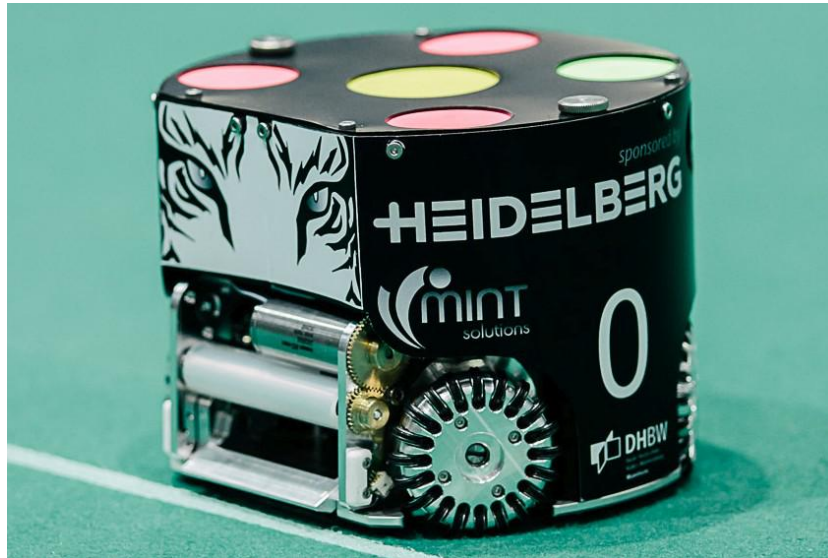
Fig. 2: New robot with cover on the field (v2016). Left and right to the dribbling device the new infrared barrier protection can be seen (white).
