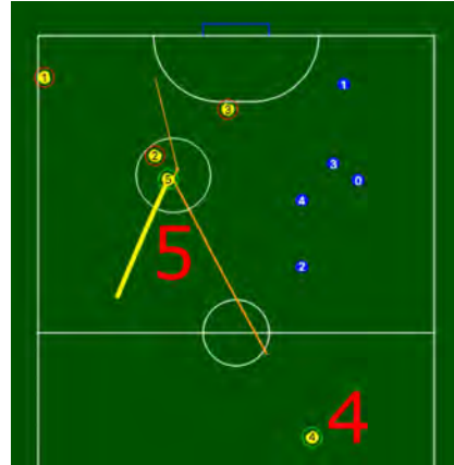
(b) Robot 5 has adjusted its trajectory in order to intercept the ball successfully, kicking it towards the goal.
