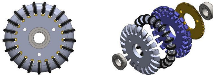
(a) New type omni-wheel with 21-discs (b) Components of the omni-wheel
