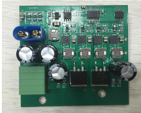
Fig. 7. Demo Board of New Power Supply Subsystem
