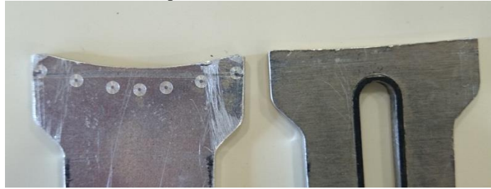
Fig. 1. Shape of kick bar (left one is newer)
