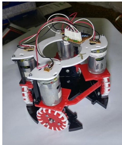
Image 4: Support Ring Mounted onto Athlete chassis
