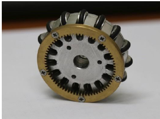
Fig. 6 Inside view of our Omni-Wheel
