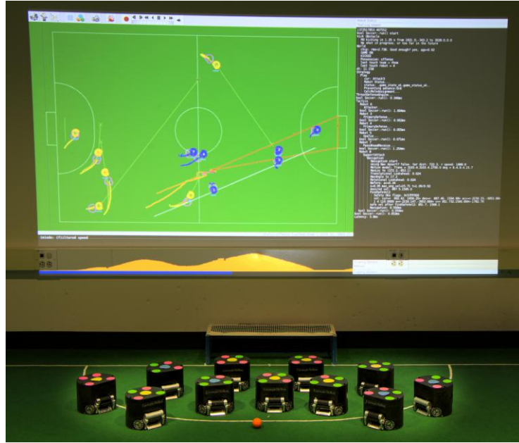
Fig. 1: CMDragons team of soccer robots. In the background, our layered disclosure viewing and debugging tool [4].
