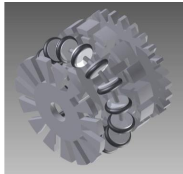
Image 2: Omni Wheel Exploded View
