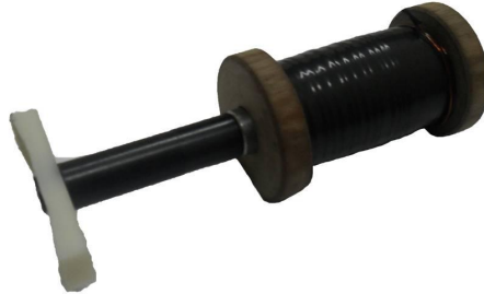
Fig. 5. Picture of the STOx's flat kicker. It provides a maximum kick speed of 10m/s
