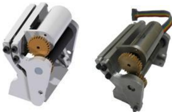
Fig. 4. Dribbling System. The top of the dribbler device contains both the cylindrical rod and the brushless motor to keep the ball from moving forward when the robot moves. The left Figure shows a computational model of the dribbler. The right Figure shows the actual implementation of such design.
