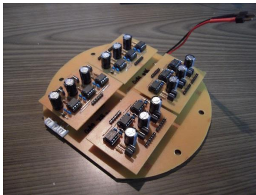
Fig. 5. The Motor Driving Circuit Board
