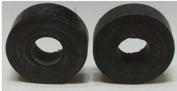
Fig. 7 Small tire of polychloroprene, before experiment (left) and after that (right)
