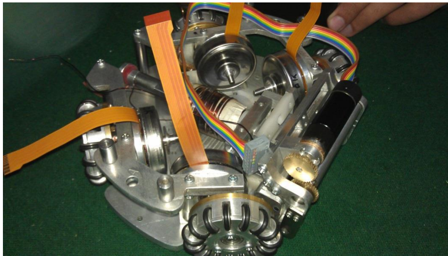
Fig 3.3 Complete Assembly with Dribbler Mechanism
