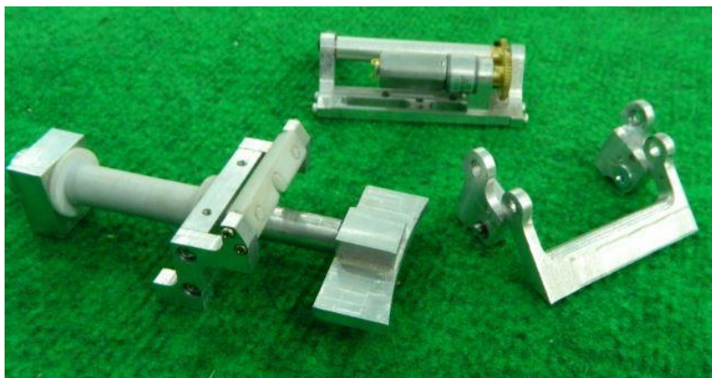
Fig.3 (From Left to Right), Kicker Assembly, Dribbler assembly, Chip Kick Assembly
