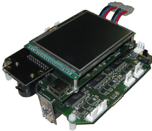
Fig. 2: Mainboard with mounted TFT, camera and wireless module
