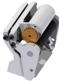
Fig. 4. Model of the dribbling system
