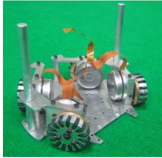
Fig. 2. Robot's chassis with wheels and motors
