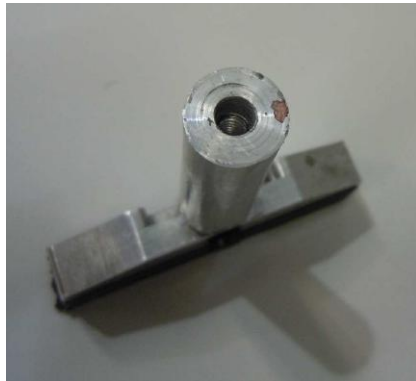
(a) Kicker plunger thread failure
