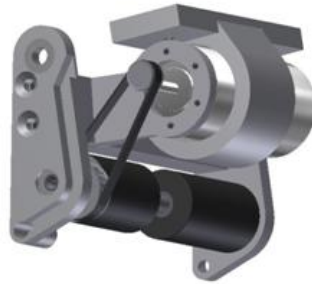
Fig. 2. Dribbler and damper system showing the belt and pulleys connecting the motor to the dribbler bar
