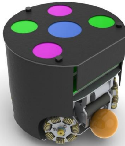
Fig. 1. Render of the previous (pre-2012) shield design. The side is attached to the top with a fragile bead of epoxy which is prone to failure.
