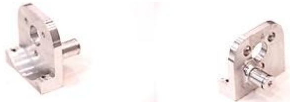
Figure 19: Motor stands with modifications on the shaft and chassis connecting surface
