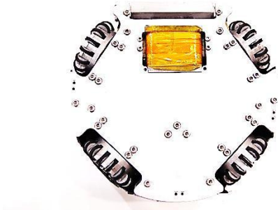
Figure 20: Robot new chassis with added stands' screws.
