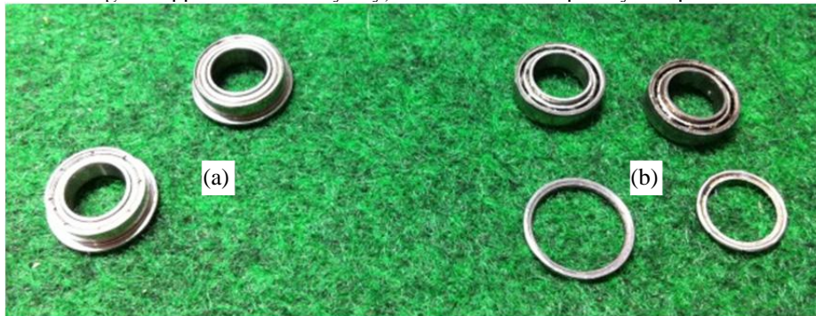
Fig. 2 Bearings used in wheel of 2011 version, (a) normal and (b) broken
