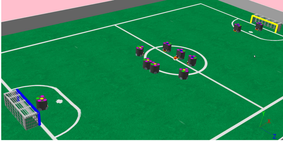
Fig. 8. Simulated ssl environment in Webots. Robots have exactly the same number of rollers in the omniwheels, and they can kick the ball as well as dribble although these behaviors haven't been developed yet.
