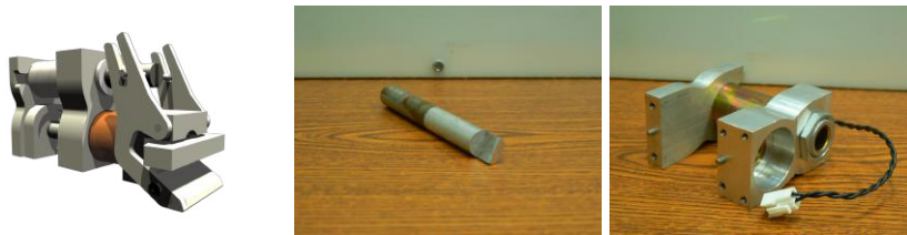
Fig. 5: Kicker & Chipper Rendering (left) vs. Plunger Bar (center) vs. Kicker & Chipper Mounts (right)
