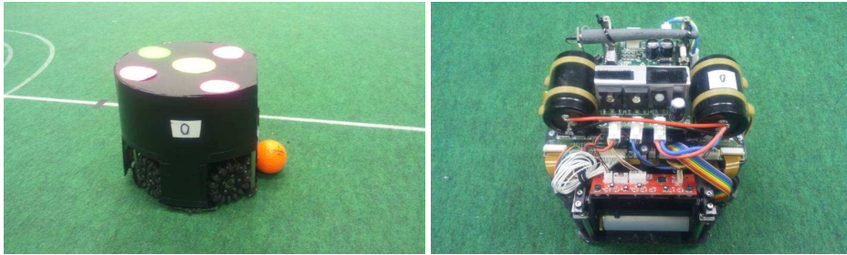
Fig. 2. Current Robot (Left: with cover and ball, Right: without cover)
