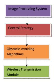
With the help of coordinates of the robots, their orientations and the ball's coordinates given by the vision system, Control Strategy determines the best way for the robot soccer team to react. It uses AI in the task, to manipulate a complete strategy for the team that optimizes the results.
