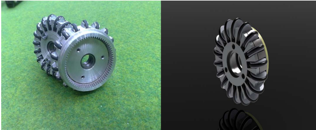
Fig. 5. Wheels of (Left) MRL2010, (Right) Designed wheels for MRL2011
