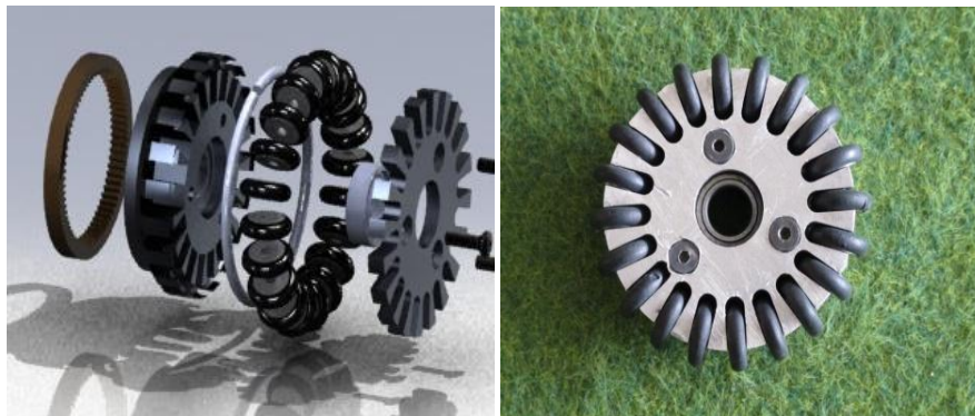
Fig. 28. Wheels for MRL2011 (Left) Designed in Solidworks, (Right) Produced wheel image
