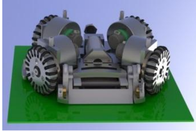
Fig. 29. Mechanical main body, including the motors, wheels, and both kickers.
