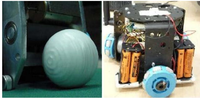
Fig. 2. Test robots. Left, Dribbling system. Right Final robot
